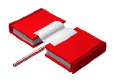
Investigation: Place the two books or folders parallel to each other on a table and approximately 3" apart. Then, place the sheet of paper over the gap between the books, with the edges of the paper resting on the inside edges of the books. Using the straw, blow underneath the paper as hard as possible. The paper will be pushed down in the middle toward the table.
