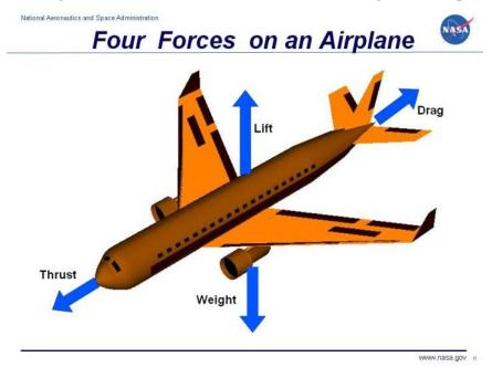
Explain the difference between the forces of lift and weight and thrust and drag.
